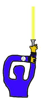
The arm with a wrist mounted compass is held across your body in front of your line of sight and the compass window indicates the bearing. Now holding the torch parallel to the bearing, you can use the beam to pick out your path along the floor.
