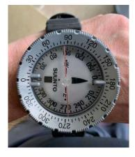
**Coming Back** – you have a choice to reset the compass to the back bearing of  $265^{\circ}$  or leave it set at  $85^{\circ}$  and simply turn around until the North arrow on the gimble is pointing at the South (single peg) on the bezel. Lubber line still reads  $85^{\circ}$  but is  $180^{\circ}$  out.
