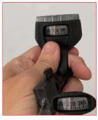
**Back Bearing** – turn until the window shows 265°. Choose suitable objects to navigate to as waypoints on the return swim. A simple slate can be used to help plan more complicated routes. Sports divers can plan a very simple out and back navigation. Dive leaders should plan a more challenging exploration with options for divers who are short of air or bottom time. A Capenwray Challenge is included for you to test your skills – see 'navigation challenge'. First more on Waypoints.
