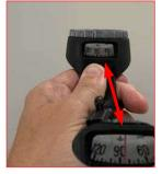
Compass held at arm's length. Turn until the sighting window reads 85° and this is the direction we intend to travel. Simple.
