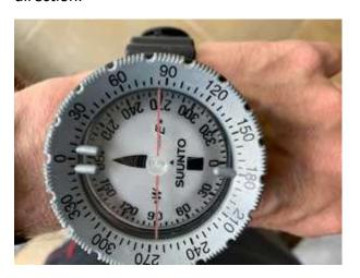
**Sense Check** – North is 360° and 0, therefore 85° should be roughly East – see bezel! Other side of lubber line gives back bearing.
